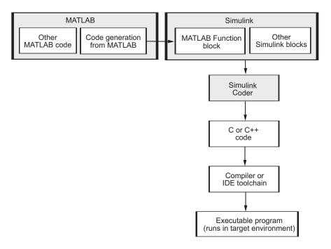
The code generation workflow is a part of the V-model on page 1-4 for system development. The process includes code generation, code verification, and testing of the
